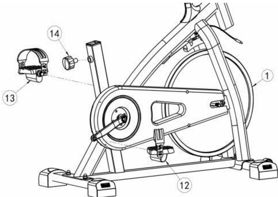
Install the right pedal (12) with R mark on The Main Body (1) and fix it with an open wrench (25). Note: tighten it clockwise.
