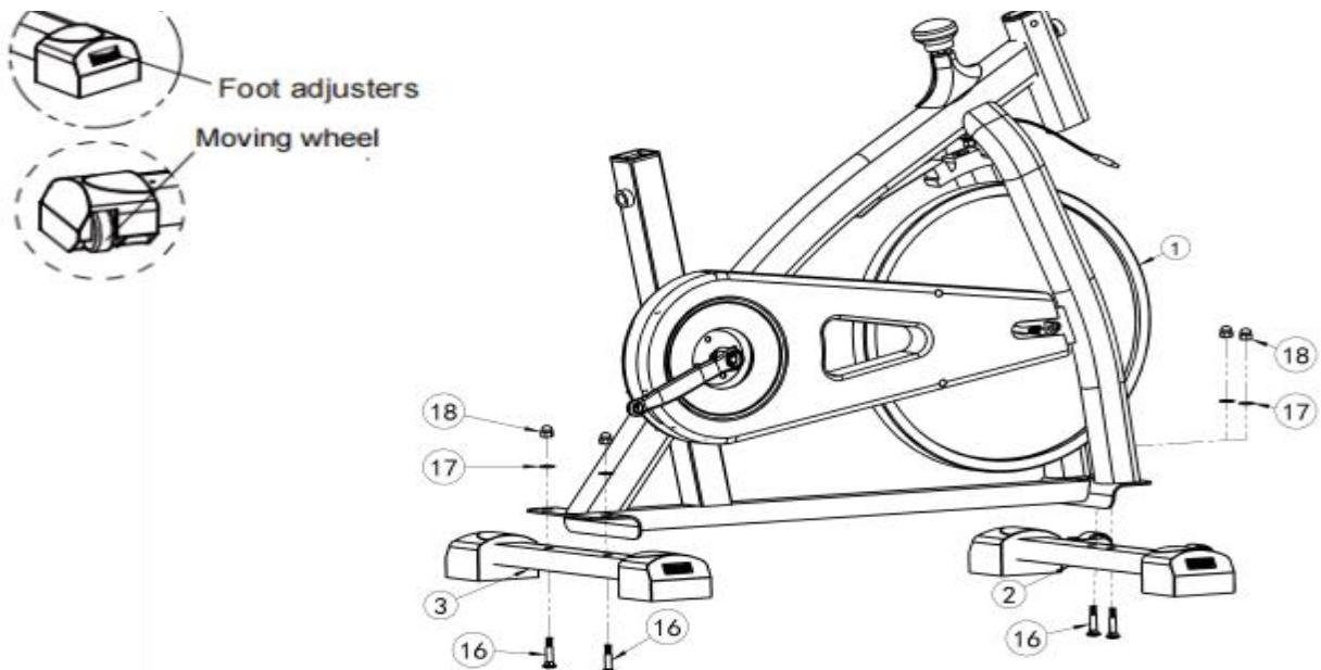
The Front Stabilize (2) is fixed on the Main Body (1) with Carriage Bolts (16), Flat washers (17) and cover nuts (18), and fixed with open wrench (25). Note: the move wheels of the Front Stabilize(2) are forward,as shown.
