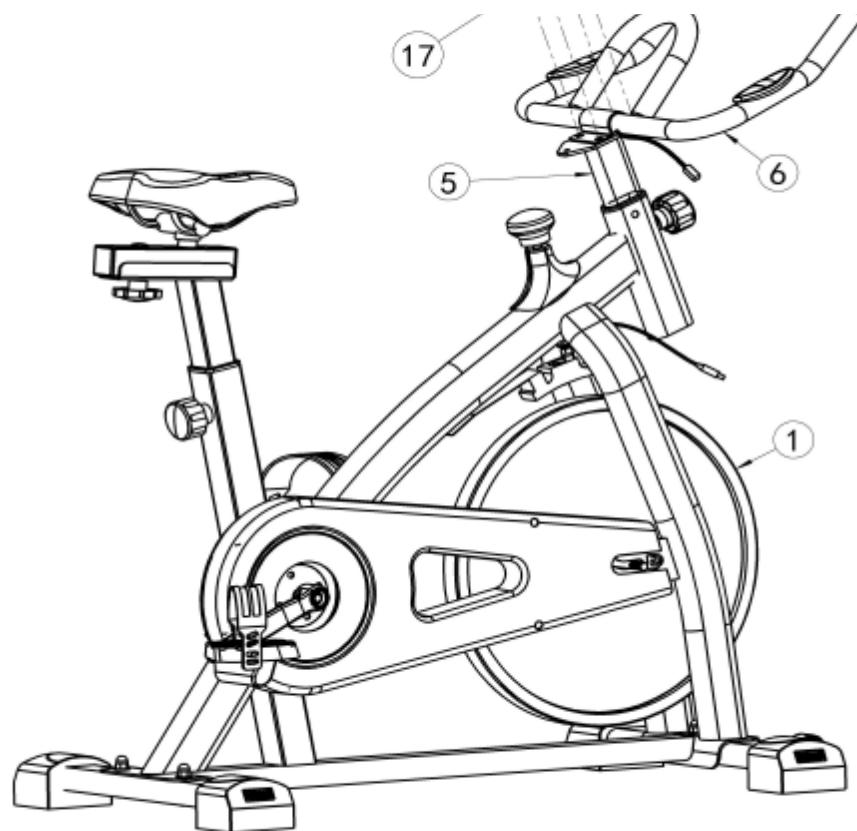
The Handle Frame (6) is fixed on the Handle Post (5) with Flat washers (17), the Spring washers (21) and the Button head bolts (20), and tightened with an inner hexagonal wrench (27).
