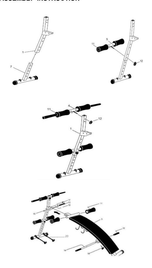
Connect the Main Frame(2) to the Upper Support Frame(1) using one Hexagonal Bolt (13) ,Lock Nut (15) and Washer(19) , the insert the Safety Pin(17) , Attach the Cross Bar(14) Using one Locking Knob(18).Moisten the inside of the Foam Grip(10) & Circular Foam Grip(11) with household furniture polish( liquid) spray and slides onto both ends of the tube, finally place Pull Rope (20).
