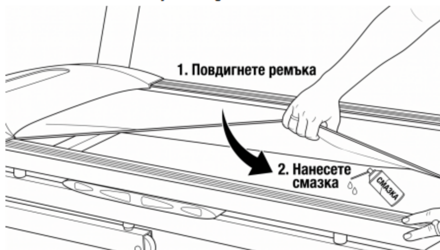
Lubrication diagram. Labels in the original diagram: 1 — lift the belt; 2 — apply lubricant.
