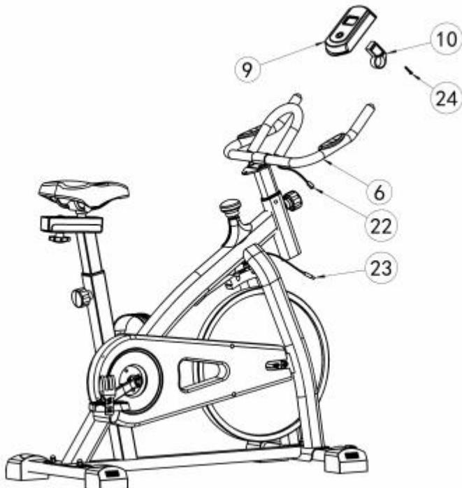
The Monitor Holder (10) is pulled and fixed on the Handle Frame (6) with the Self tapping screw (24) and tightened with the inner hexagonal wrench (27).
